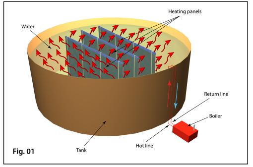
Showing how Endura-Form panels can be used in flat panel assemblies for heating and cooling large volumes of materials and can be used below ground. Multiple assemblies can be used. In the image shown here, three panel sections are used to heat a large tank of water. A glycol solution is used for heating.
