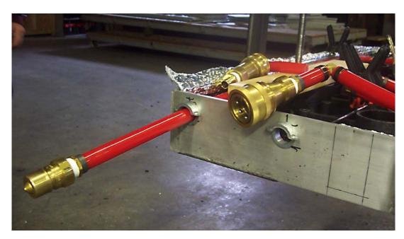
**Figure 11**: This shows the male and female quick connectors. The right hand line has not yet been run through it's port. The quick connectors would attach to the external heat lines which would carry the glycol heating fluid to and from the heating source. The heating source will vary from application to application.
