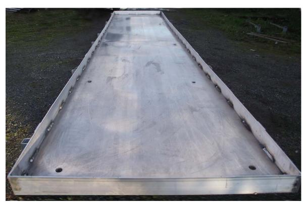
**Figure 01**: This shows the assembled aluminum tray that with hold the Endura-Form panel assembly. This framework gives the assembly great rigidity and strength allowing it to be easily handled and it can be placed on blocks or stands if needed. The has 4" x 1/4" aluminum angle with a 1/4" aluminum sheet is welded to the bottom. Drain holes are fitted at regular intervals to allow melt water to drain away. The solid bottom also gives protection from any surface the walkway may rest on.
