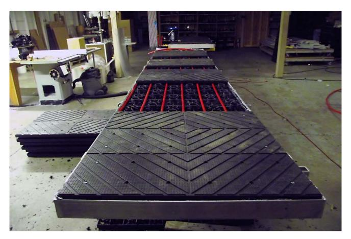
**Figure 14**: This shows the top layer partially assembled - you can see the half panel at the near end that gives the panels their interlocking offset. A few bolts are alsi in place.
