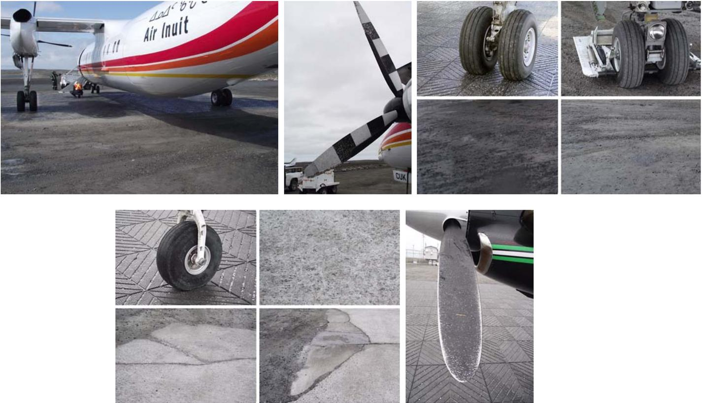
Compare the Endura-Form apron with the normal gravel runway and how much cleaner and easier it is to maintain. The propellers in the center pictures show the damage running on a bare gravel or dirt runway can cause. Endura-Form panel installations can help prevent this sort of damage.
